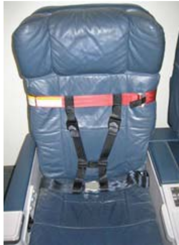
FIGURE 10. EXAMPLE OF A CRS (ACSD) APPROVED THROUGH STC AND UNDER § 21.305(d) (2010 ed.)
