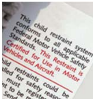
FIGURE 3. EXAMPLE OF REQUIRED LABELING
