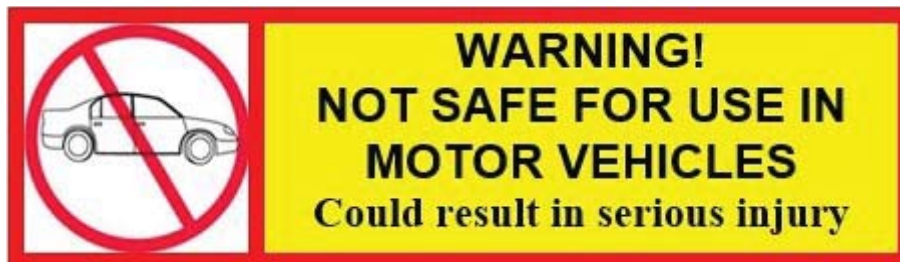
FIGURE 2. REQUIRED WARNING LABEL FOR AVIATION CHILD SAFETY DEVICES WITHOUT FMVSS NO. 213 APPROVAL
